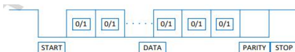
Figure 12 LPUART data transmission format
